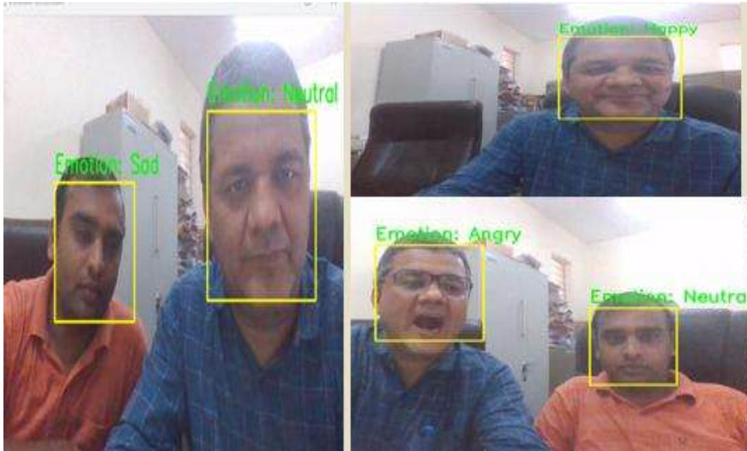
Figure 4.12: (from Left to Right) Testing Result Sad and Neutral expression by Proposed System Testing Result Angry and Neutral expression by Proposed System Testing Result Happy expression by Proposed System
