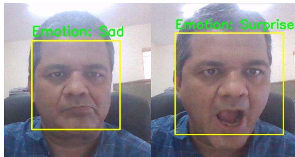
Figure 4.9: Testing Result of Sad and Surprise expression by Proposed System
